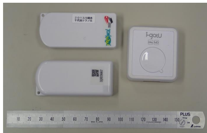
Figure 1. Personal dosimeter “D-shuttle” (left) and GPS logger (right) used in the study
