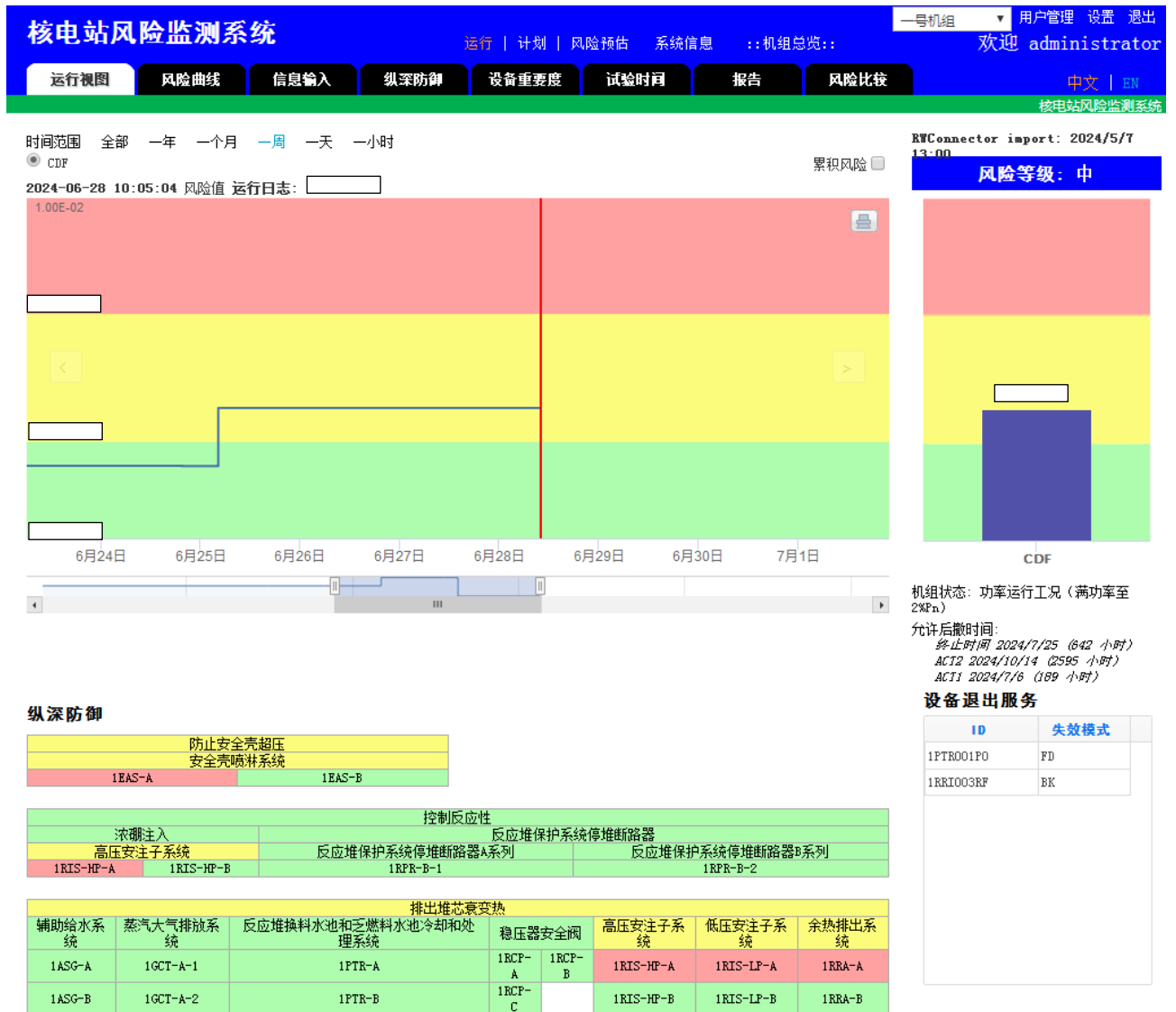
Figure 2. Operator Screen for Operational CRM with ACT values
