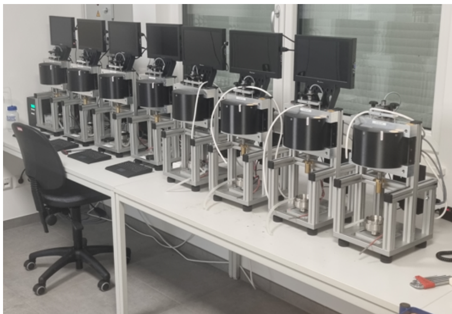
Figure 3. New developed fully assembled test rigs for fatigue tests of dental implants (Heß et al. 2024)
