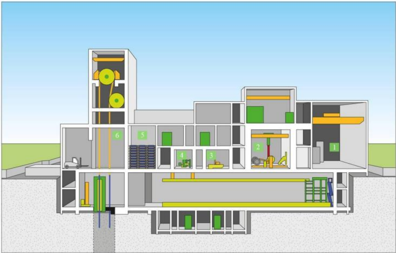
Figure 1. Encapsulation plant. Reception of fuel and storage of the transport cask (1), fuel handling chamber (2), copper cover welding station (3), weld inspection station (4), reception and storage of empty deposition canisters (5) and canister lift (6) (Ahlbom, 2021)
