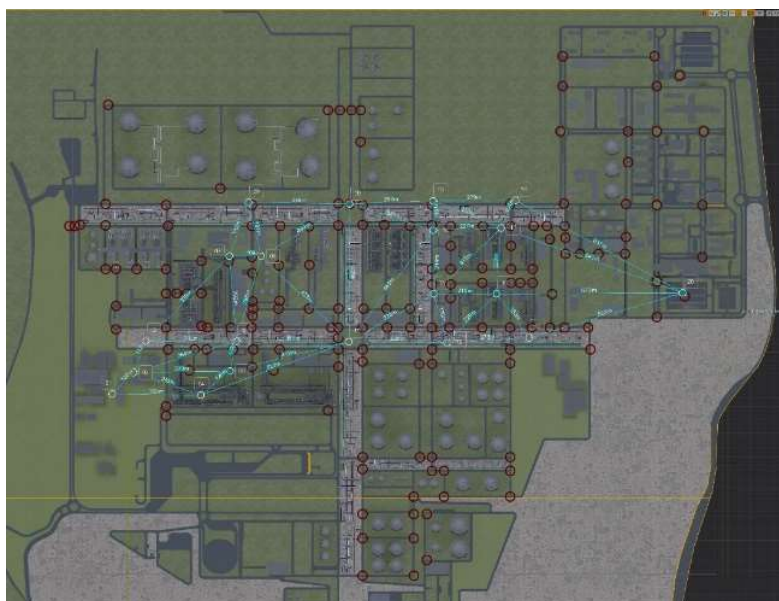
Figure 7: Smart sensors placement in all plant, superimposed on the original grid. Source: The Research.
