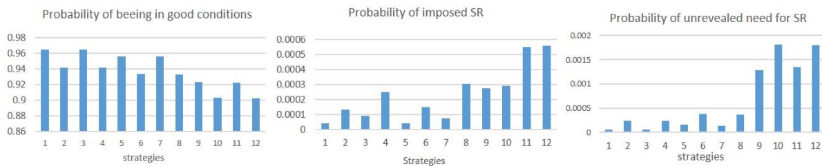
Figure 10 Probabilities of good conditions (left), speed restriction imposed (centre) and unrevealed need for speed restriction (right).
