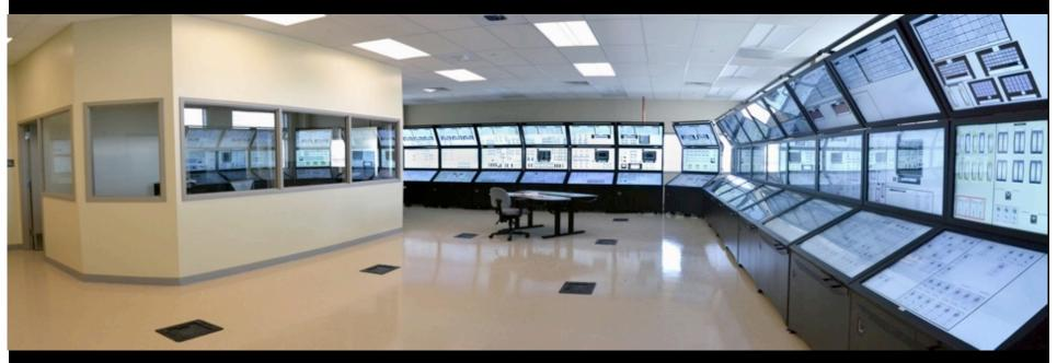
Human Systems Simulation Laboratory a reconfigurable, full-scale, full-scope research simulator to support NUREG-0711 activities
