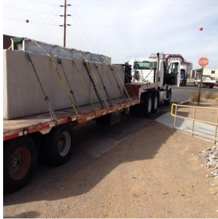
Figure 15: Surrogate assembly on 38 mile Truck transport. The assembly is bolted and strapped to concrete blocks to simulate the weight of a transport canister. (photo: Saltzstein)
