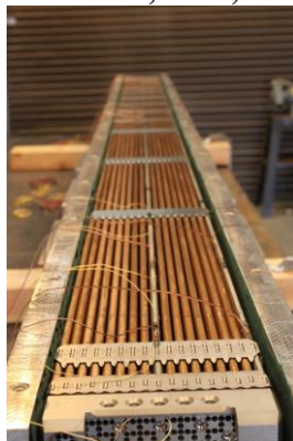
Figure 11: The surrogate fuel assembly instrumented with accelerometers and strain gauges. (McConnell, et al., 2013)
