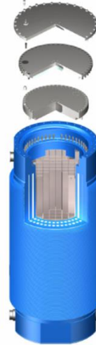
Figure 1: Major characteristics of dual purpose casks (pictures: Castor ® V design by GNS mbH)
