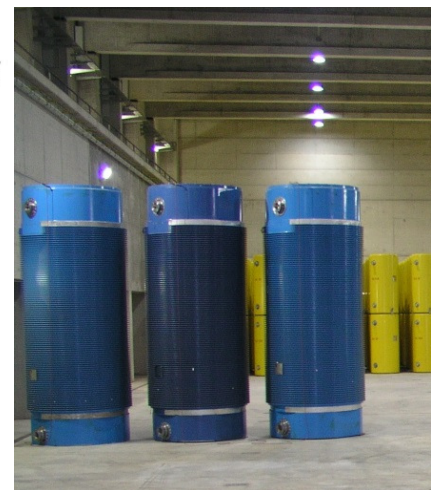
Figure 2: CASTOR ® V/19 casks in transport cask storage facility Ahaus (Photo: GNS)
