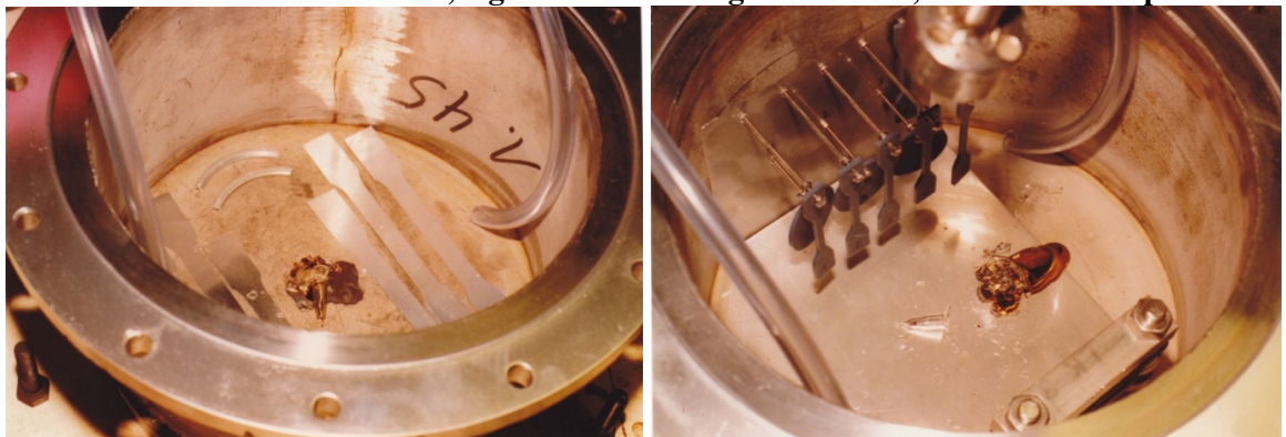
Figure 5: Aluminum (left) and Silicon rubber specimen (right) prepared in flasks with exposure of 5 g Cesium; Cesium released from a destroyed glass ampoule on the bottom.
