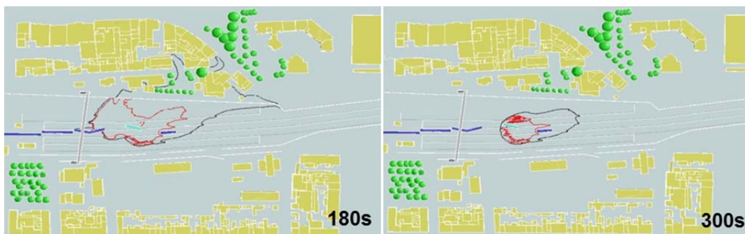
Figure 4: LFL (black) and UFL (red) footprints at 180 and 300 seconds for 5D E-NE atmospheric conditions and a wall 2.5 m high on the east side
