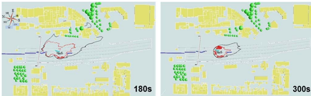
Figure 2: LFL (black) and UFL (red) footprints at 180 and 300 seconds for 5D E-SE atmospheric conditions
