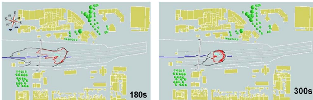
Figure 5 LFL (black) and UFL (red) footprints at 180 and 300 seconds for 5D W-SW wind atmospheric conditions and a wall 2.5 m high on the east side
