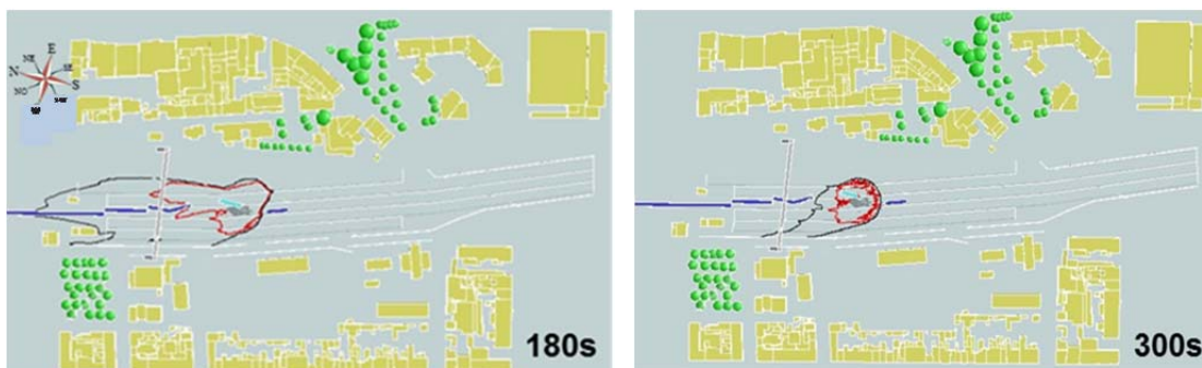
Figure 3: LFL (black) and UFL (red) footprints at 180 and 300 seconds for 5D W- SW atmospheric conditions
