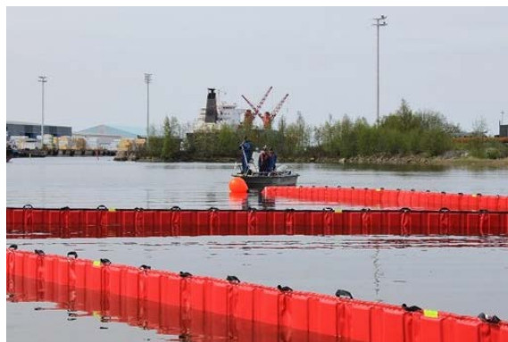
Figure 6. A deployed oil boom in the Kalajoki harbour. [8]
